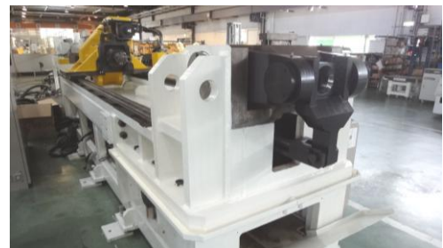
Pipe-Multibender exclusive for work pieces with round cross-section
